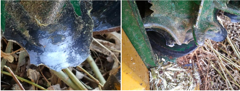
Figure 18 Wear on cutting knives of JF 192
